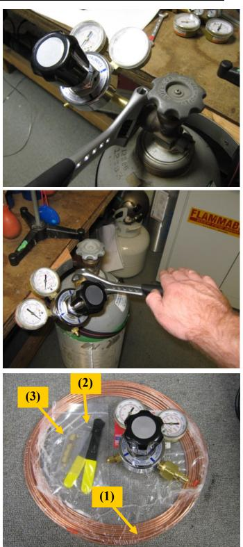
Cut the copper tubing to the desired length using the tubing cutters and secure the nuts and ferrules to both ends of the tubing (see our *Cutting Tubing* and *Using Ferrules* documents for more information). Stainless steel 1/8" tubing can also be used, but it is harder to cut and more expensive than copper tubing.
