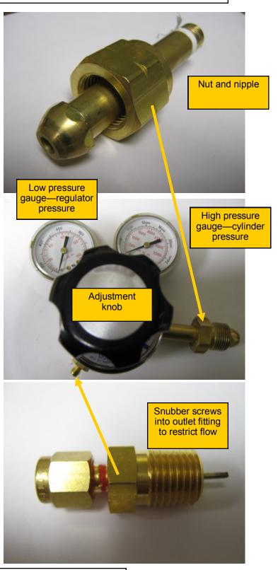
To tighten the gas regulator onto the cylinder first ensure that the CGA fitting is the proper one for the given cylinder of carrier gas. This number is usually stamped on the metal valve at the top of the cylinder and also on the nut and nipple. Flammable gases tighten up in the reverse direction.
